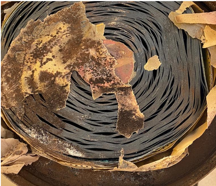
Plate 1: Decayed acetate film showing high level of deterioration Source: NFVSA, Jos.
