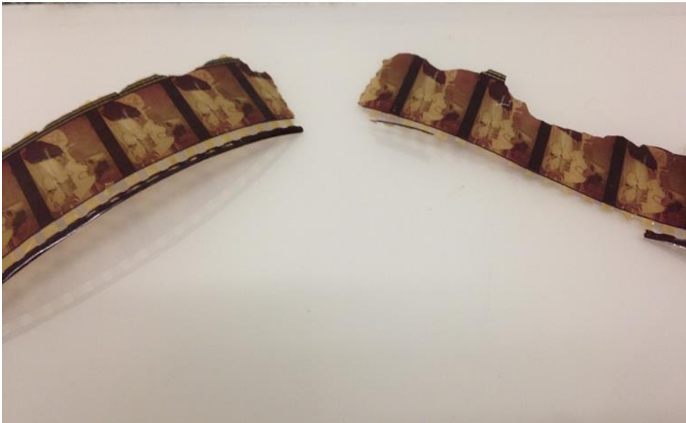
Plate 3: Shaihu Umar film strip showing various damages and colour fading Source: Arsenal Institute for Film and Video Art, Berlin.
